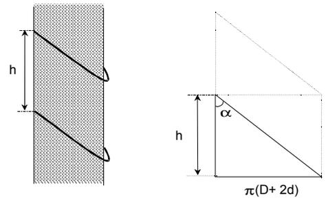
FIGURE 5 WEAVING STEP PARAMETER
