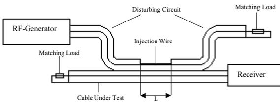
FIGURE 2 CURRENT INJECTION TEST SET UP
