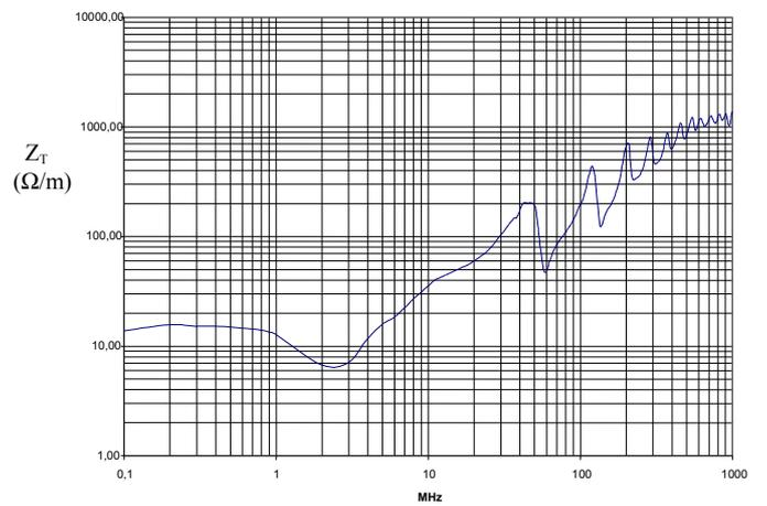
FIGURE 6  $Z_T$  MEASUREMENT RESULTS (MTREK2700)
